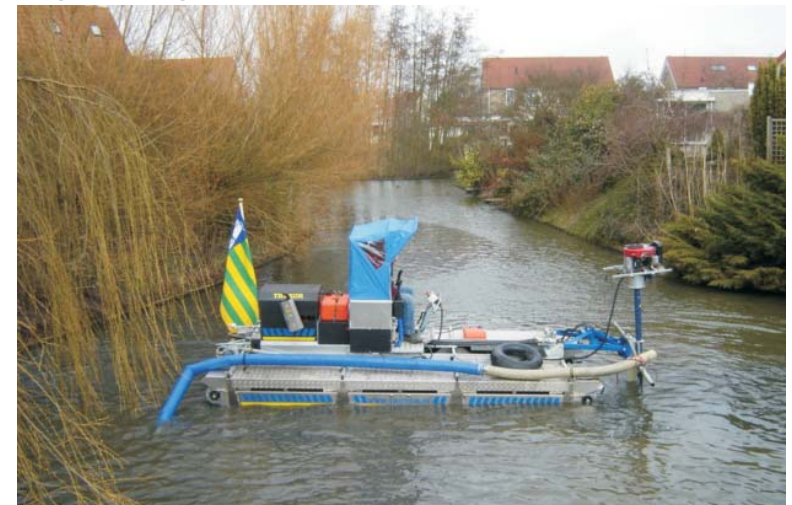
Dredge pump MB-LL80 B-4 A dredge pump for dredging slurry from ponds and other water areas. Specially designed to fit on the lift arm of the MOBITRAC
